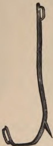
FIGS. 232-233.—Eastern pole climbers, with and without strap for attaching to legs.
